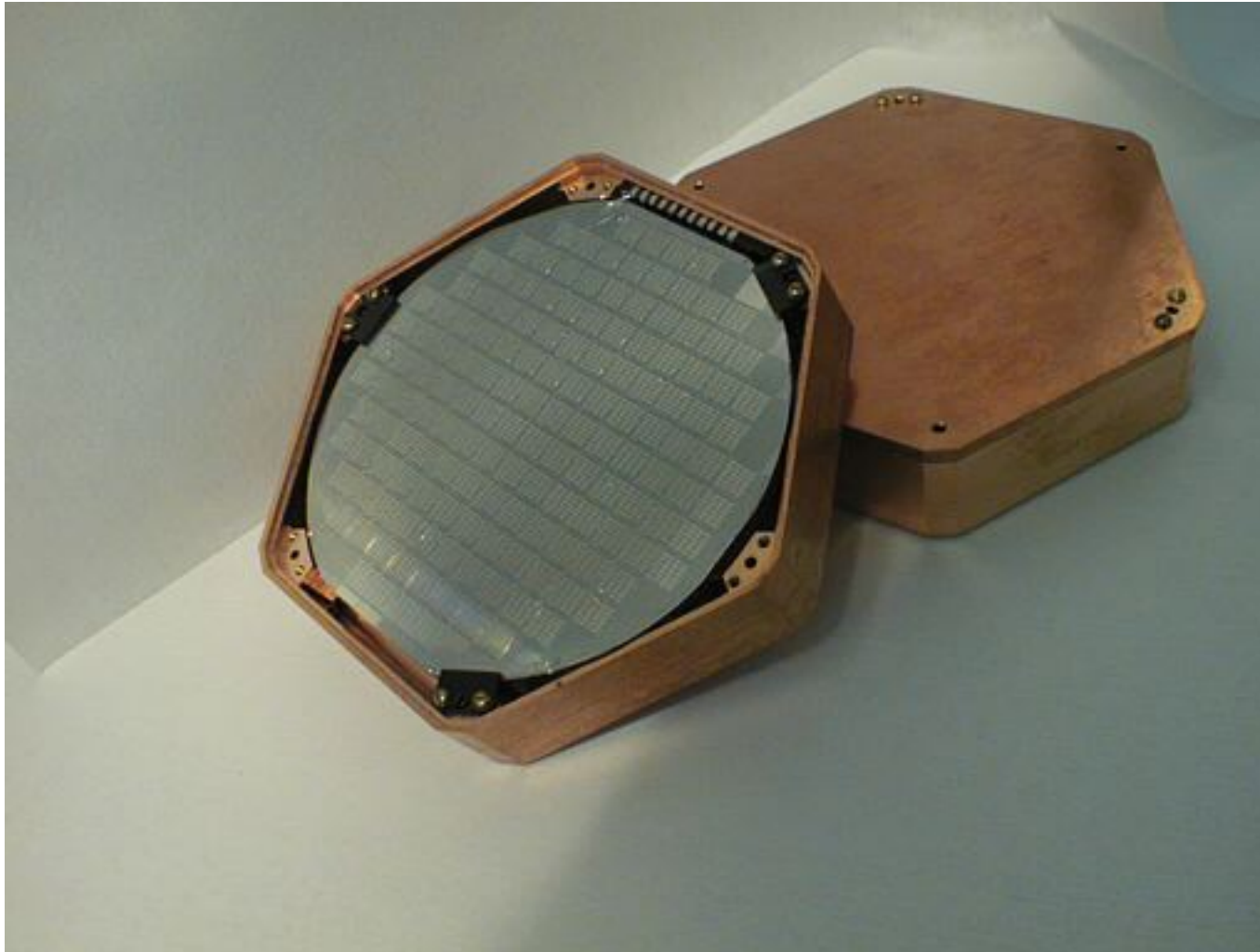
CDMS detector. Operates at 40 mK
